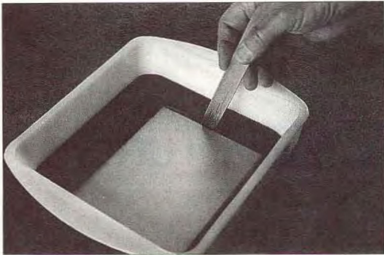
Photo C. The circuit board floating on the etchant. A stick is used to lift the board momentarily to purge bubbles.
