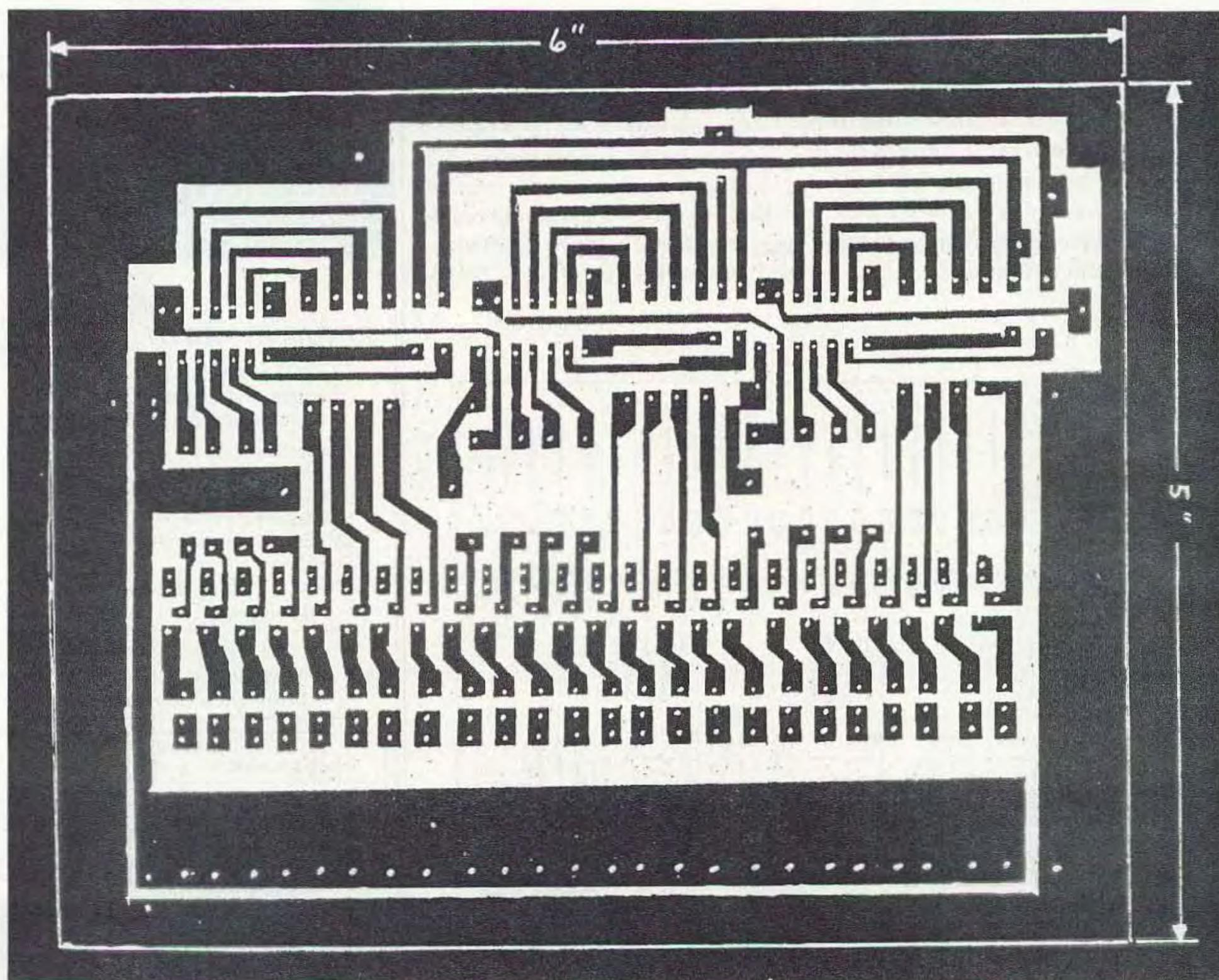
Fig. 4. PCB top foil side.
