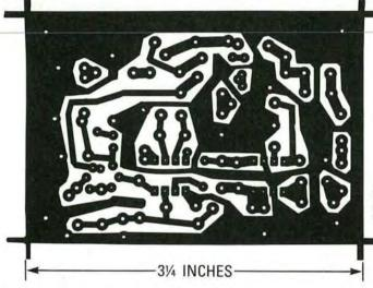
USE THIS PATTERN to build a descrambler for the outband system used by some cable-TV systems.
