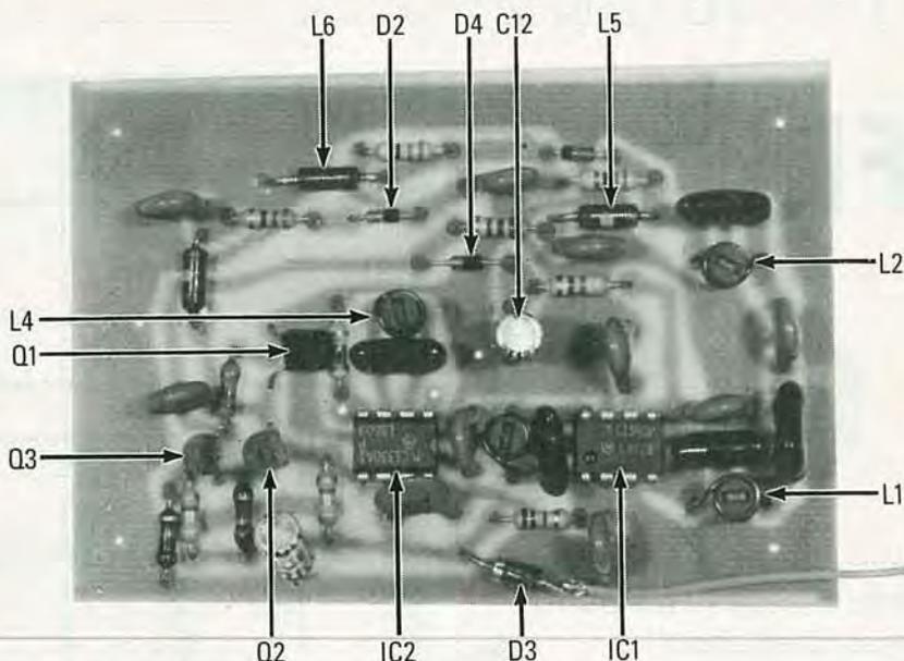
FIG. 8—THE FINISHED OUTBAND DECODER is shown here.
