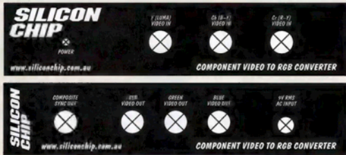
Fig.7: these full-size artworks can be used as drilling templates for the front and rear panels.
