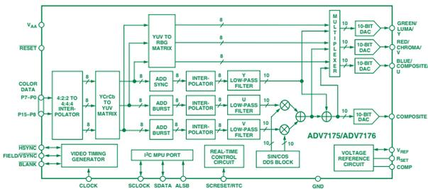
The output circuitry enables the part to support the ubiquitous standard composite video formats as well as the increasingly popular performance S-Video (Y/C) video mode. The four outputs mean that the part can simultaneously drive a variety of combinations of CVBS and S-Video. For example:
