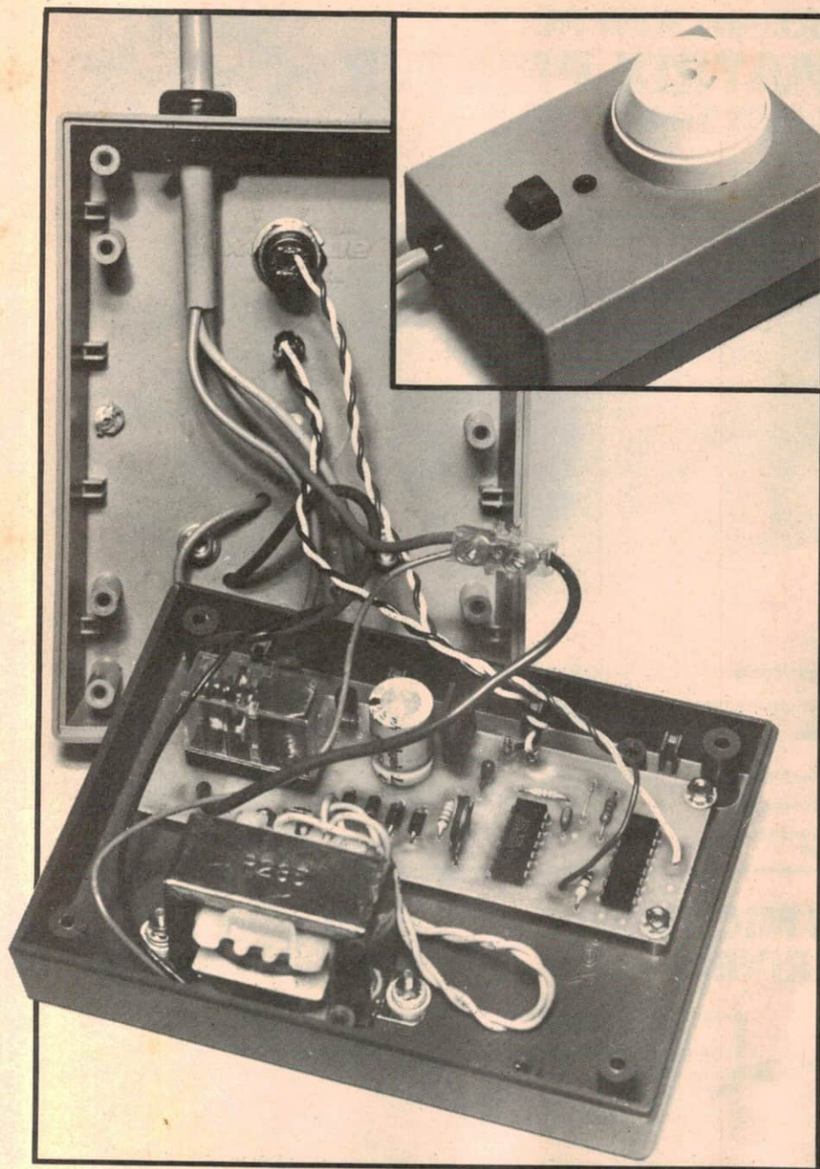
▲ On the inside. Showing construction of the project and how I mounted it inside the Unibox case. Note that one of the internal pillars is cut down to provide clearance for the transformer. Inset. The completed project.
