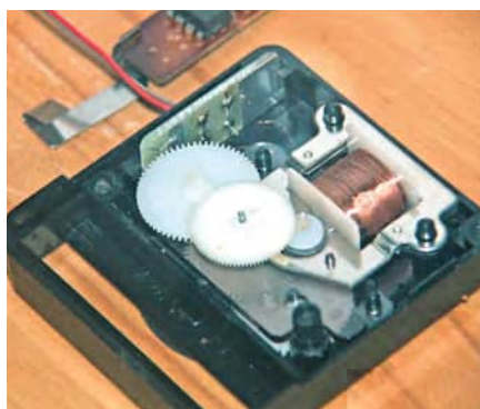
Fig.1: inside a typical quartz clock mechanism with stepped second hand, showing the modifications we made to terminate the connecting leads to the stepper motor coil.
