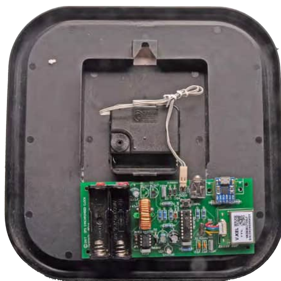
Here's how we secured the PCB to the clock – a little bit of judicious filing removed a couple of ridges, then a few dollops of silicone sealant holds the PCB securely in place. This method allows easy battery change later on.
