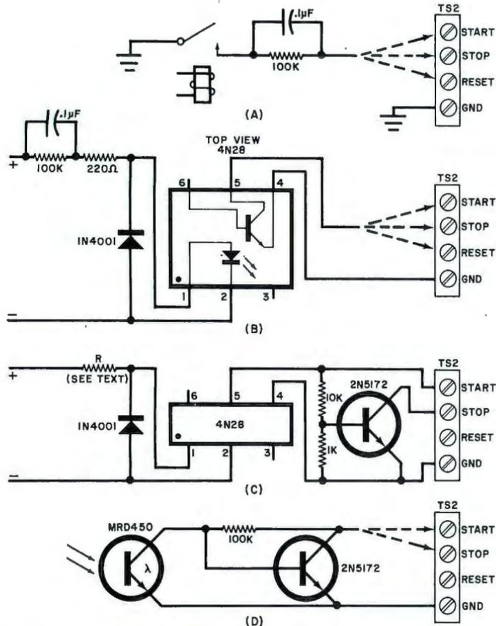
Fig. 4. Stopclock can be operated by a relay (A); an optoisolator (B and C); or a phototransistor (C).
