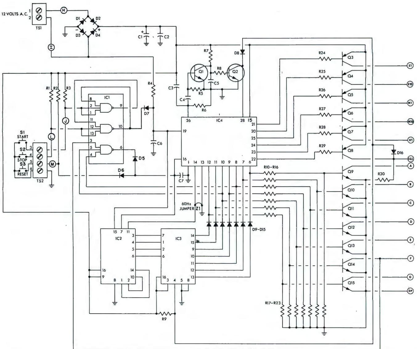
**W**OULD you like to know precisely how long a recording session runs; how long it takes to make one lap around the track; or how long that new amplifier has been cooking on the bench? Here is a new six-digit stopclock that can do it—counting and displaying elapsed time up to ten hours by tenths of a second.
