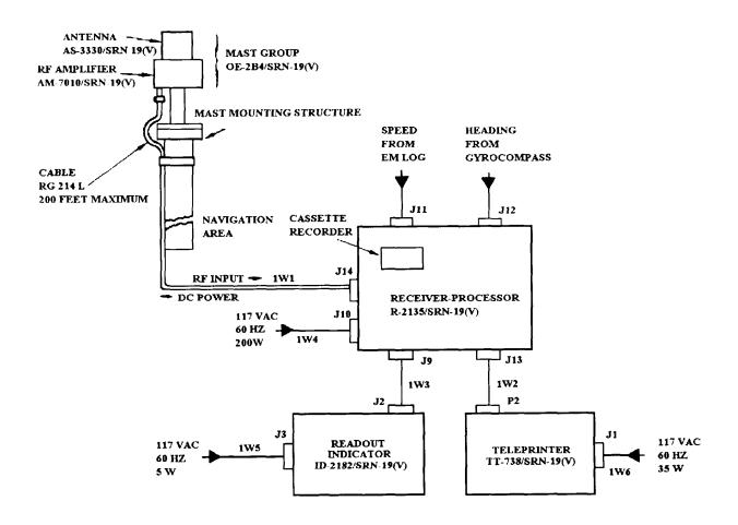
Figure 1-10.—AN/SRN-19(V)2 simplified block diagram.
