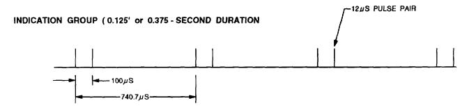
Figure 2-4.—Transponder output pulse train.
