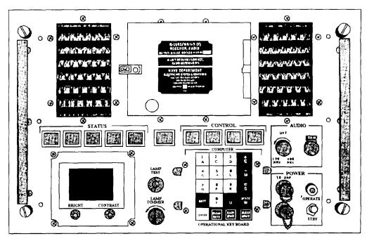
Figure 1-8.—AN/WRN-5 front panel.
