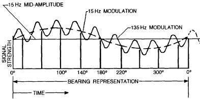
Figure 2-6.—TACAN modulation envelope
