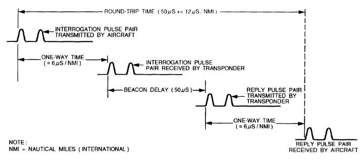
Figure 2-2.—Distance measuring round-trip travel time.
