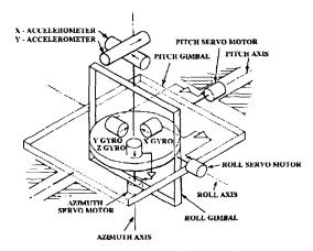
Figure 1-1.—Stable platform with inertial components.
