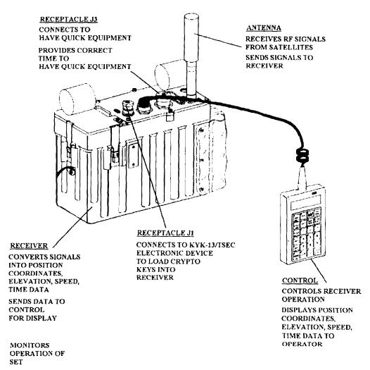
Figure 1-14.—Manpack Navigation Set AN/PSN-8().
