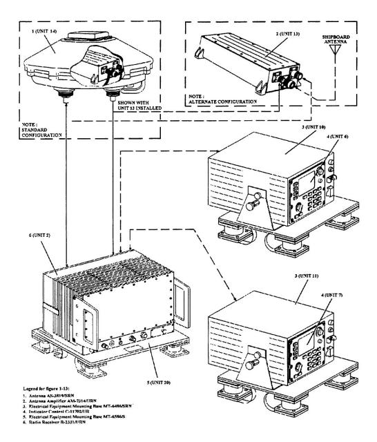
Figure 1-13.—Satellite Navigation Set AN/WRN-6(V).
