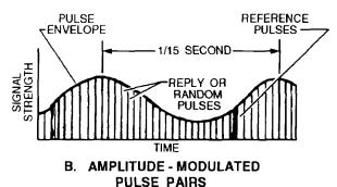
Figure 2-5.—TACAN radiation pattern: A. cardioid pattern; B. Ampltitude-modulated pulse pairs.
