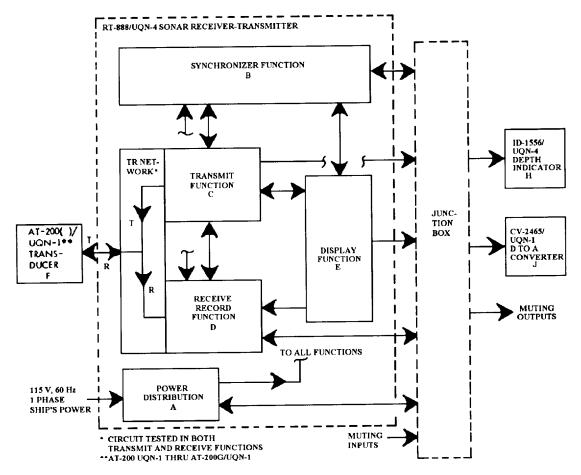
Figure 1-15.—AN/UQN-4A functional diagram.
