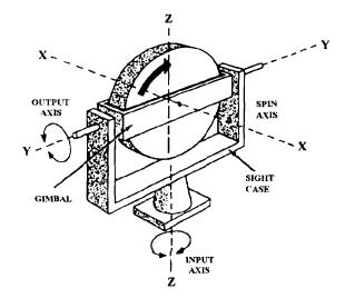
Figure 1-4.— Gimbal-mounted rate gyro.
