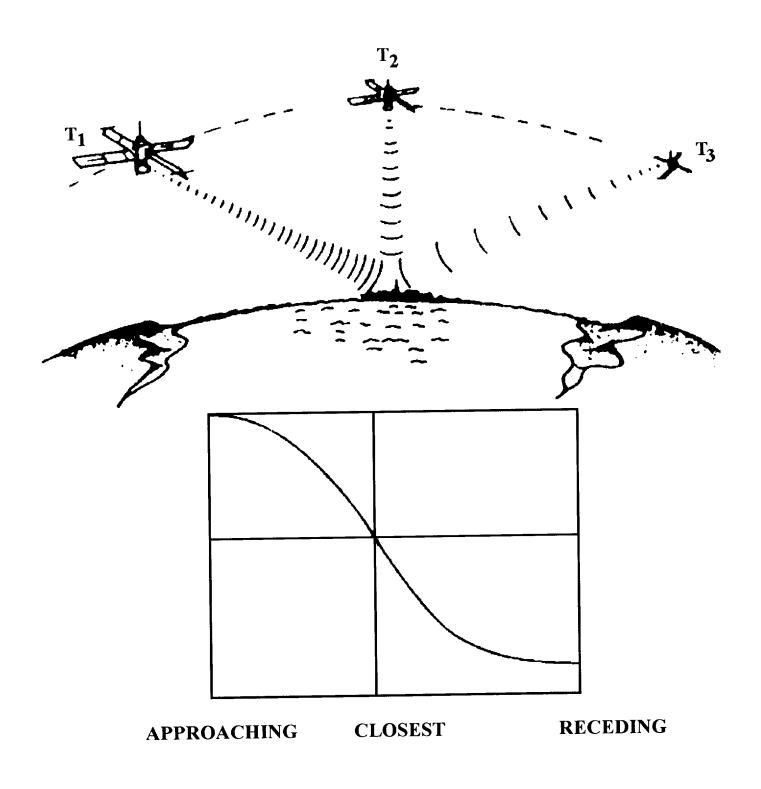
Figure 1-7.—Doppler shift relative to satellite transmitted frequency.
