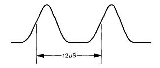
PULSE WIDTH =  $3.5 \pm 0.5 \mu$ S PULSE RISE TIME =  $2.5 \pm 0.5 \mu$ S PULSE FALL TIME =  $2.5 \pm 0.5 \mu$ S
