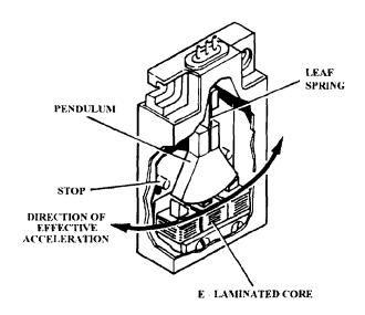
Figure 1-2.—E-transformer accelerometer.
