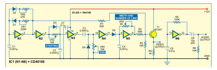
pattern generator on the TV screen help you align the vertical scanning synchronisation circuit of the receiver.
