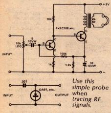
This simple two-stage audio amplifier with volume control has several applications. It can be used as a general purpose amplifier to amplify the output of such things as crystal sets; it can be used for tracing signals in audio circuits; and, when coupled to a suitable probe, can be used for tracing modulated RF signals.
