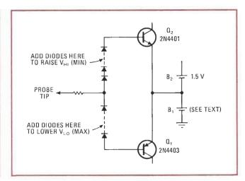
**2. Setting the gap.** Circuit of Fig. 1 can be modified by addition of diodes to change the maximum voltage for "boop" tone,  $V_{L0}(max)$ , and/or the minimum voltage for "beep" tone,  $V_{HI}(min)$ . Any silicon diodes can be used; the voltage drop is about 0.5 volt per diode at the low diode currents.
