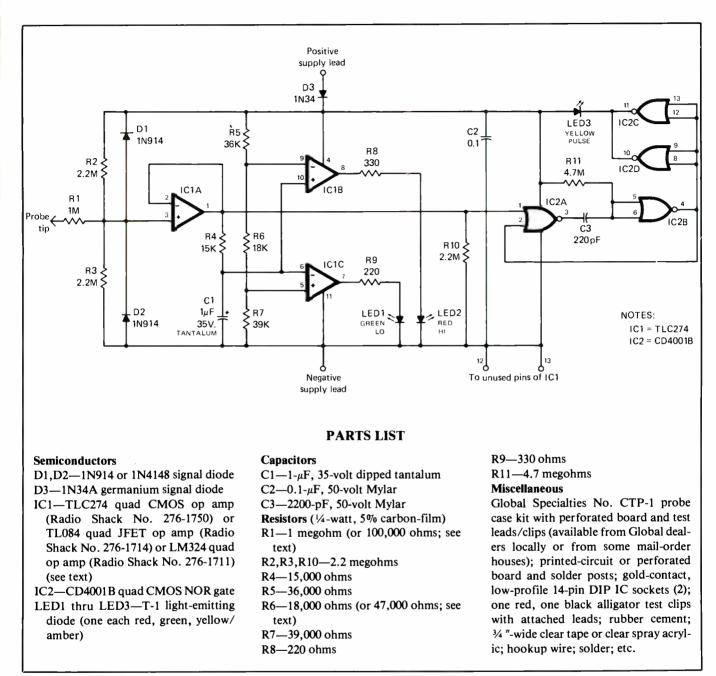
Fig. 1. Note in this overall schematic diagram of the Looker digital logic probe that only three of the four operational amplifiers in IC1 are used. The fourth op amp is disabled
