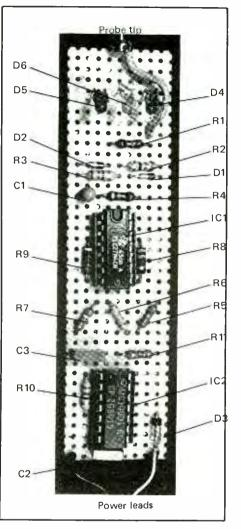
Fig. 3. This is the recommended layout for the parts on the perforated board supplied with the probe case kit. Note the unusual mounting of the LEDs. Use sockets for the ICs.
