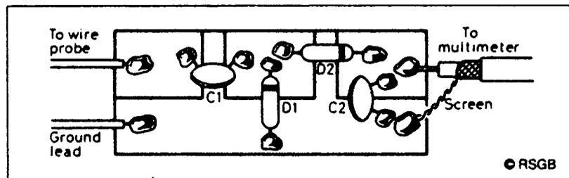
its base, being careful *not* to touch any of the components. Connect the croc clip to a ground point on the circuit and touch the probe on the circuit point to be tested. If an RF signal is present, there should be a reading on the multimeter. That's all there is to it!
