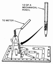
of a mechanical pencil or ball-point pen with a metal cartridge. A needle is forced into the tip of the pencil or pen. The test lead is thin coax cable with its core soldered to the pencil tip (the positive prod) and the shield (the negative lead) is soldered to the body of the compass at the top. Connectors on the other end of the cable match your meter.—Peter Legon
