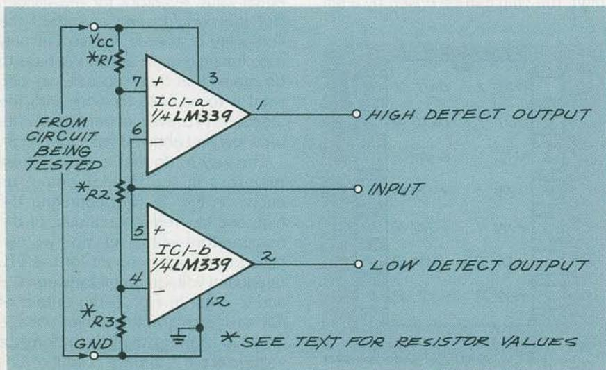
**FIG. 2**—IN THIS LOGIC-PROBE CIRCUIT we've tied together one pin from each comparator. Those pins will receive the input voltage from the probe. The low detector is inverting and the high detector is non-inverting.
