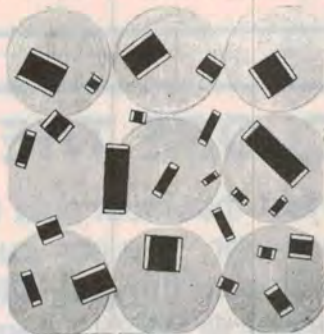
Figure 3. Ceramic chip capacitors — shown about actual size. They have no leads, just plated end pads for connections.
