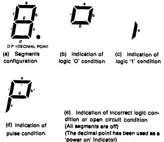
Fig. 1: Segments configuration and the resultant indications obtained.
