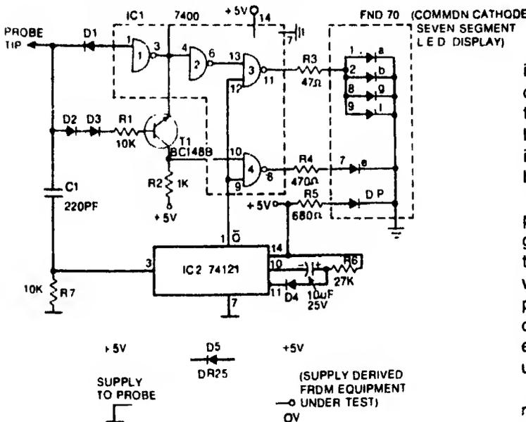
inactive. Diodes D2 and D3, transistor T1 and gate 4 form the circuit that detects logic one condition. D1, D2 and T1 ensure that for all voltages between 2V and 5V the logic one circuit becomes active while for voltages below +2V it remains inactive. Thus, for voltages greater than 0.8V and less than 2V both the detecting circuits remain inactive.
