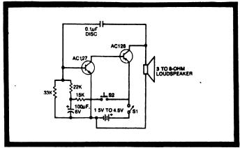
Wiring is not critical, and the entire unit can be constructed on a small piece of PCB or groupboard.
