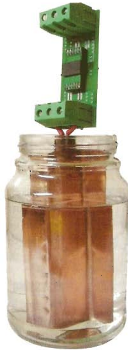
Fig. 2. Electrochemical dummy load cell consists of two parallel plates or electrodes placed in a jar containing an electrolyte.
