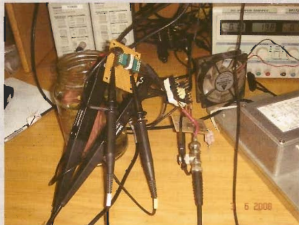
Fig. A. The connection of the various measuring probes onto the transformer.
