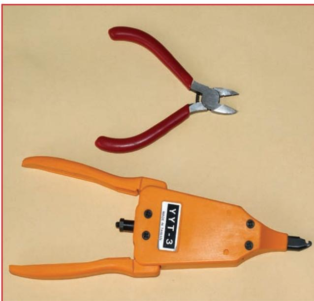
Fig.2. The spring-loaded wire cutters (bottom) and the conventional type (top) will both do the job well, but the conventional type is all that is really needed for electronic project work
