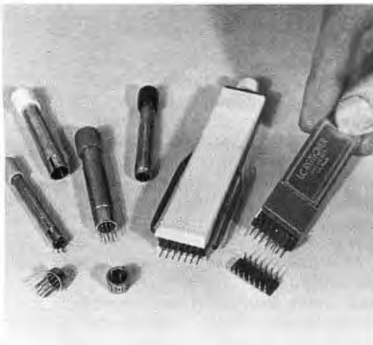
GC Electronics Quick Pick Tools (left) and IC remover (right), with Pul-N-Sertic semiconductor inserter and remover (center)—all very handy.
