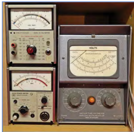
Fig.7.27. Part of the author's RF test bench showing a variety of RF voltage and power meters purchased from second-hand dealers and from on-line auction sites
