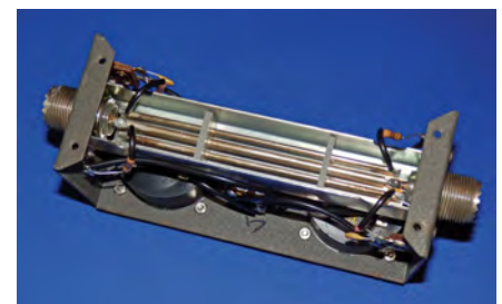
Fig.7.19. The interior of an HF SWR bridge showing the main transmission line and the two coupled transmission lines that feed the forward and reverse detectors
