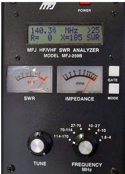
Fig.7.22. HF/VHF antenna analyser for operation between 1.8MHz and 170MHz. The instrument can display resistance, reactance, impedance, reflection coefficient and SWR
