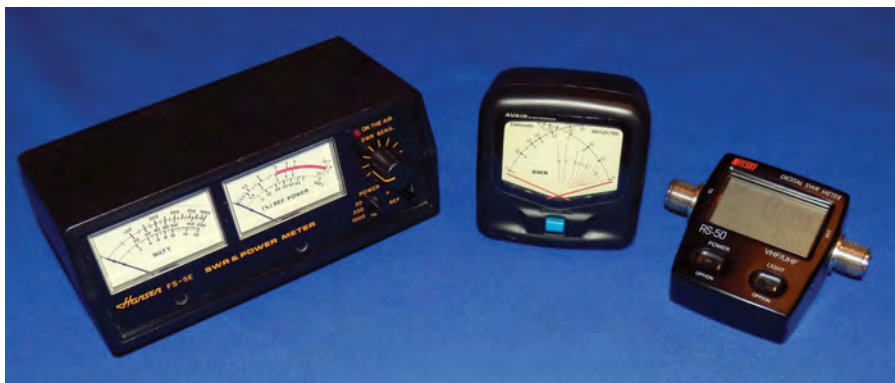
Fig.7.18. Typical low-cost combined RF power meters and SWR bridges
