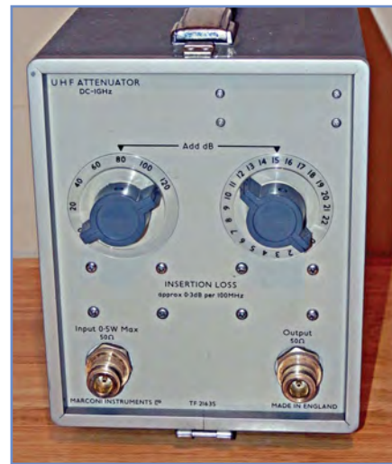
Fig.7.30. A Marconi switched attenuator suitable for use from DC to 1GHz with attenuation of up to 142dB in steps of 1dB
