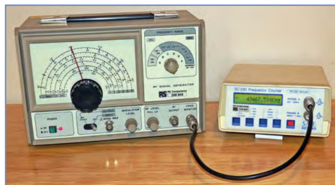
Fig.7.12. Bench test instruments: an RF signal generator used with a digital frequency meter (DFM)
