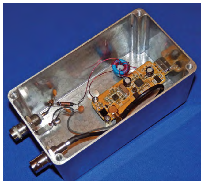
Fig. 7.15. A DVB-T tuner 'dongle' modified to support MF/HF as well as VHF/UHF inputs. This permits operation over a frequency range extending from around 100kHz to well over 1GHz
