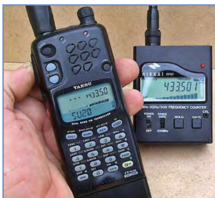
Fig.7.11. Checking the output frequency of a dual-band FM transceiver. The digital frequency meter (shown on the right) indicates a frequency difference of 1kHz
