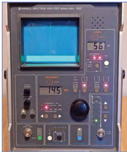
Fig.7.29. A Farnell 352C spectrum analyser suitable for use from 300kHz to 1GHz
