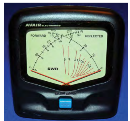
Fig.7.26. A cross-needle SWR meter (like this instrument from Avair) can be a useful investment if you need to measure RF power or adjust antennas at HF and VHF
