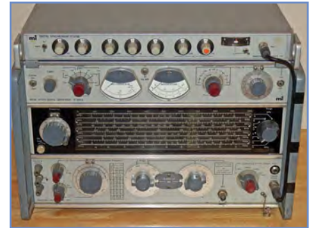
Fig.7.24. A highly accurate RF signal generator that incorporates phase locked digital frequency entry
