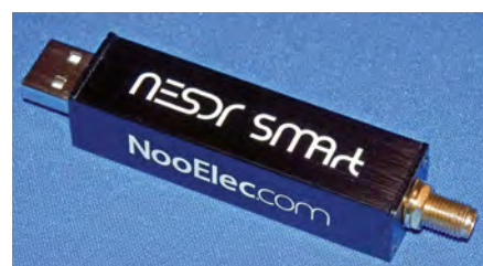
Fig. 7.14. A low-cost DVB-T tuner 'dongle' can make the basis of a simple RF spectrum analyser
