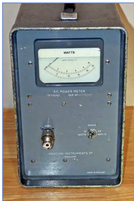
Fig.7.28. A Marconi TF1152 power meter suitable for continuous power of up to 25W with an internal load rated for use up to 500MHz. Instruments like this can make an excellent second-hand purchase
