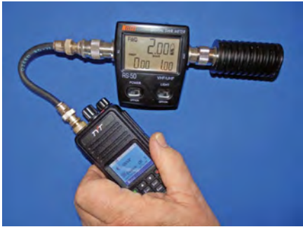
Fig.7.5. Measuring the output power from a hand-held digital transceiver (the power meter indicates an output of exactly 2W delivered to the 50Ω load attached to the power meter)
