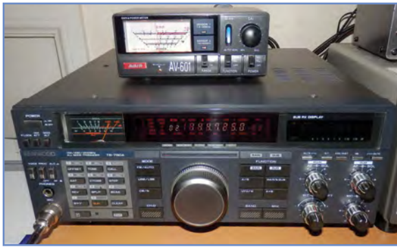
Fig.7.20. Checking output power and antenna SWR with a dual-band VHF/UHF base station transceiver
