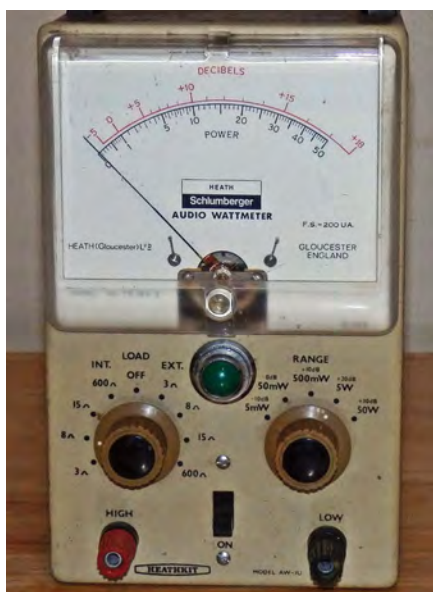
Fig.6.17. A Heathkit vintage AW-1U audio output power meter
