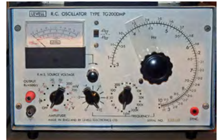
Fig.6.15. An RC oscillator with sine and square wave outputs in the range 1Hz to 3MHz, and a THD of less than 0.05% at 1kHz. Similar instruments are regularly available on-line
