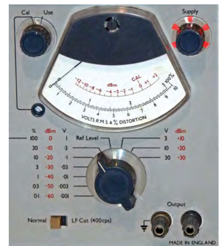
Fig.6.19. Range switch and meter calibration of the TF2331 distortion analyser (Fig.6.18)
