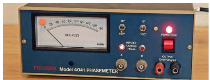
Fig.6.20. Phase meter with analogue display. The scale is calibrated from 0° to 180°, and the sign of the phase relationship (either leading or lagging) is indicated by a panel LED
