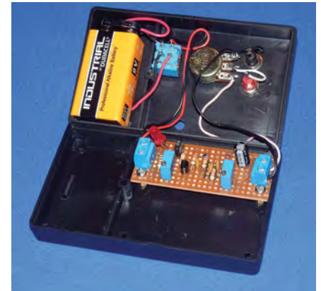
Fig.6.26. Internal wiring of the handy test signal source
