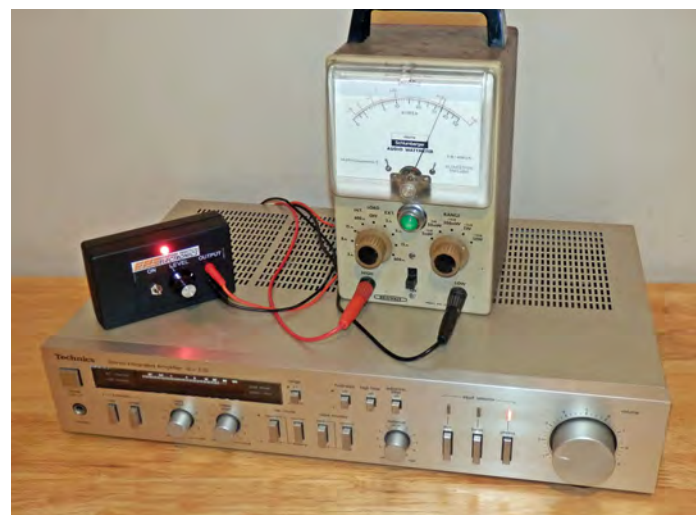
Fig.6.28. Using the signal source to test a high-quality audio amplifier at its full rated output power
