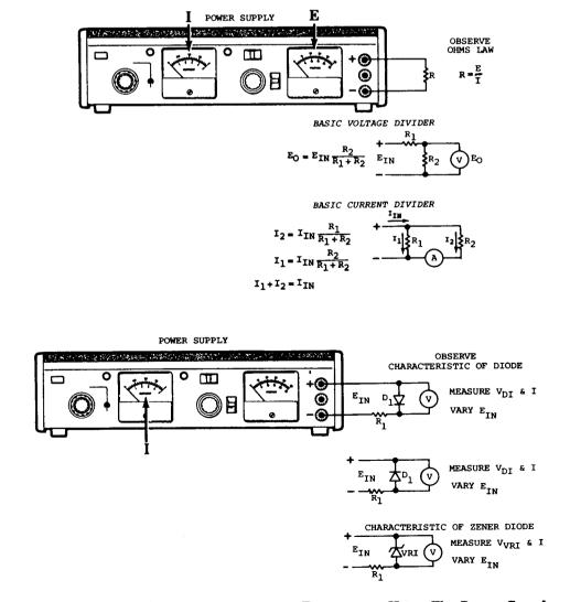
Figure 8. Typical Laboratory Classroom Experiments Using The Power Supply
