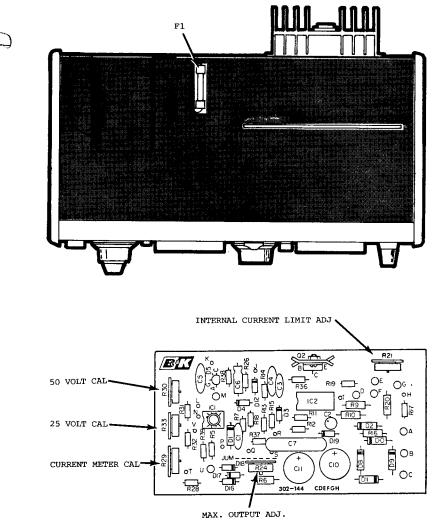
Figure 10. Location of Calibration Adjustments and Fuses
