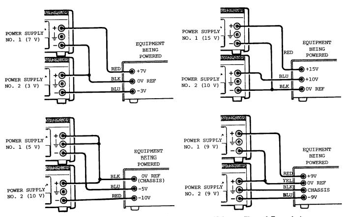
Figure 6. Using Two Power Supplies for Two Output Voltages (Typical Examples)
