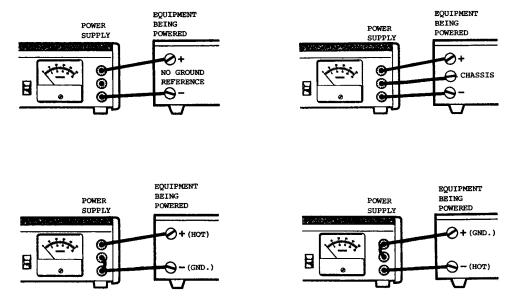
Figure 3. Power Supply Interconnect Possibilities
