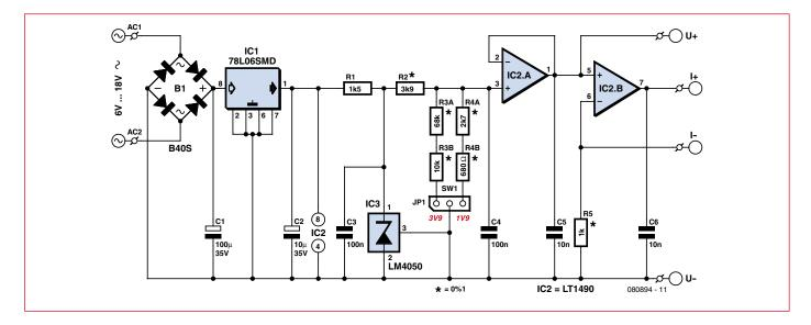
Figure 3. The volts calibrator has a voltage regulator, voltage reference, switchable voltage divider networks and a dual op amp used as a buffer and voltage/current converter.
