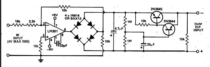
The above circuit may be used for measuring the RMS value of ac (sinewave) with a dc digital voltmeter. It has a frequency response to beyond 10 kHz and will measure signals as low '±15V, if desired, with reduce
