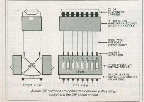
$\frac{1}{16}$ " of the free ends of each pin. Use heat judiciously when tinning and soldering pins on the DIP switches to avoid damaging their potting compounds.
