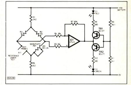
VR1. The op-amp IC1 is used to compare the two arms of the bridge. Because of this arrangement, the output level of IC1 can only be one of three values.
