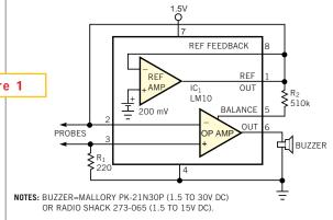
Keep an ear open for short circuits, with this easy-to-build short-circuit tester.
