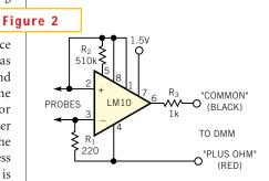
Add a short-circuit test capability to your DMM, using this modification of the circuit in Figure 1. 200 mV, which is less than the turn-on voltage for pn junctions. If desired, you can set the voltage as low as 15 mV by adding  $18\Omega$  resistance between pins 2 and 3 of IC<sub>1</sub>. However, the quiescent current increases to 1 mA.
