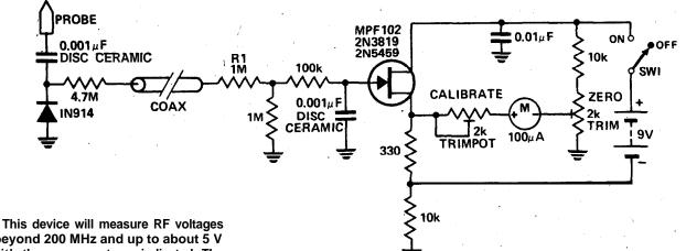
beyond 200 MHz and up to about 5 V with the components as indicated. The diode etc should be mounted in a remote probe, close to the probe tip. Sensitivity is excellent and voltages less than 1 V peak can be easily measured. The unit can be calibrated by connecting input to a known level
