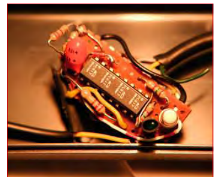
Figure 10. The PC817 quad optocoupler is by far the largest part in the PC interface.
