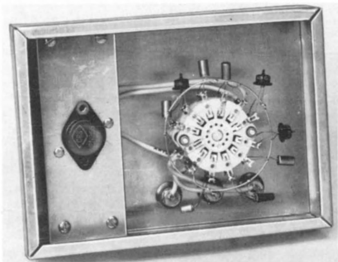
Fig. 331. Inside view of the transistor substitution box.
