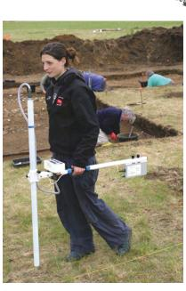
Figure 2 This field researcher is using a Grad601 flux-gate gradiometer at an archeological-dig site (courtesy Bartington).
