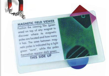
Figure 9 This viewer can directly display the presence of magnetic poles (courtesy Chen Yang).
