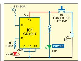
drives the LED. Flashing of the LED (LED2) indicates the presence of mains, while LED1 indicates that the scanner is active.
