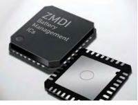
receive voltages of 4.2 to 18V and directly connects to the vehicle's battery. The IC comes in a  $5\times5$ -mm, 0.85-mm-high QFN32 package and sells for \$5.40 (low volumes). **ZMDI**, www.zmdi.com
