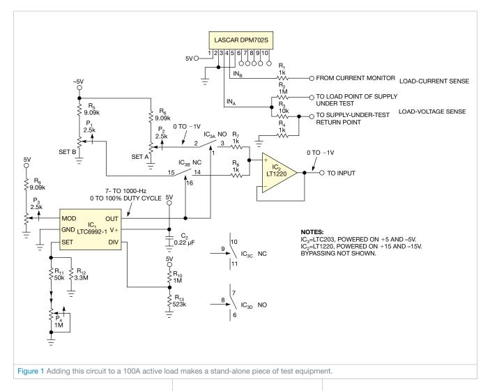
quency potentiometer,  $P_4$ . A frequency of 60 to 1000 Hz best suits use in large power supplies. You can adjust the values of the resistors to get chopping frequencies of 4 Hz to 1 MHz.
