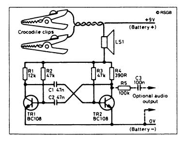
Figure 1 The circuit diagram of the continuity tester
