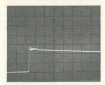
Fig. 12. After the computer-network cable in Fig. 11 is replaced with the proper type, the signal becomes much cleaner. The slow droop in the signal is caused by the capacitor-like quality of the cable: two conductors separated by an insulator.
