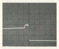
Fig. 11. A step down usually means an impedance mismatch, but the mismatch shown here is a problem of extreme proportions: using the wrong impedance cable! In this test of a computer-network cable, using the wrong type of cable results in garbled data that the interface card cannot read.
