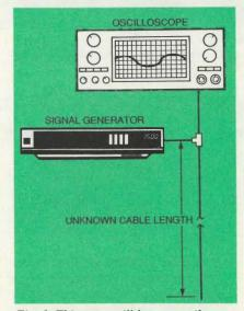
Fig. 1. This setup will let you easily measure the length of a cable without using a tape measure. Connect a signal generator to one end of the cable and measure the amount of time it takes to see the steps in the waveform on an oscilloscope.
