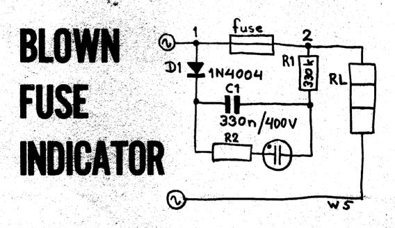
As long as the fuse is intact, points 1 and 2 are virtually shorted. However, if the fuse is blown the full supply voltage appears between these points. C1, R1, R2 and the neon lamp form a very low frequency neon oscillator. When the supply voltage appears between points 1 and 2, the neon lamp will start to flash on and off.
