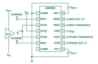
Figure 7. The AD8302, configured as a gain- and phase-comparator with controllable thresholds.
