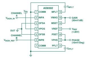
Figure 4. Absolute measurements of signal level using an AC reference on Channel B as the intercept for Channel A.
