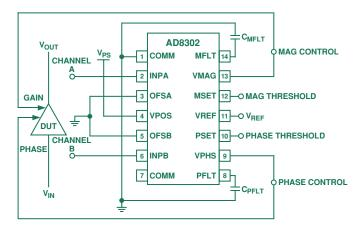
Figure 8. The AD8302 in a control loop that drives the gain and phase of a DUT towards prescribed set-points.
