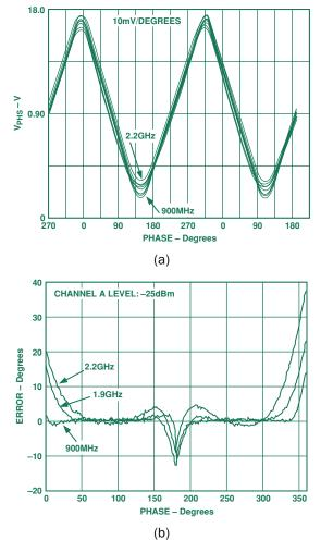
Figure 3. The phase measurement (a) exhibits low errors (b) over wide angular ranges and up to high frequencies.
