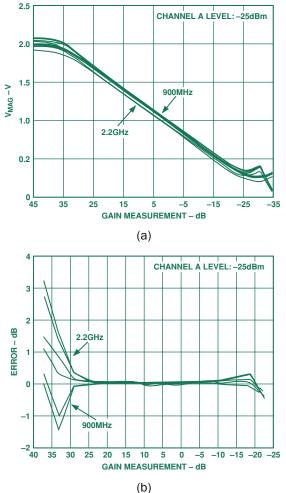
Figure 2. Measurements of signal-level ratios (a) exhibit errors (b) of less than 0.2 dB up to high frequencies.
