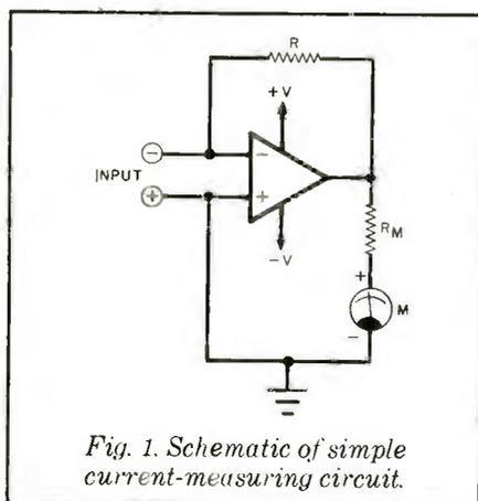
*Fig. 1. Schematic of simple current-measuring circuit.*
