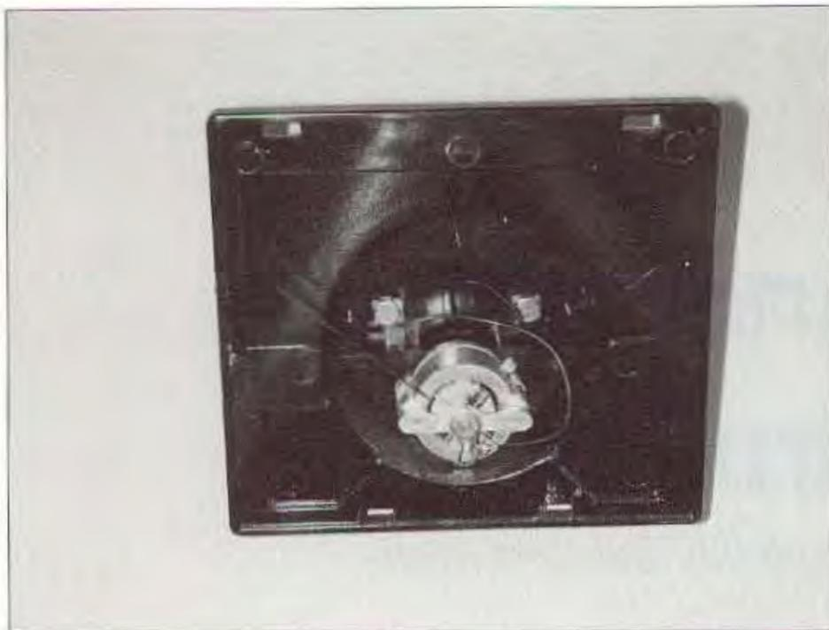
Photo C. View after disassembling meter case and removing scale plate.
