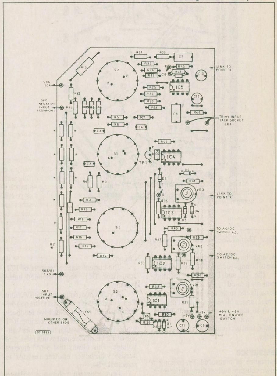
Fig. 2. Component layout on the printed circuit board. Note that the long link wires should be made with plastic insulated connecting wire.
