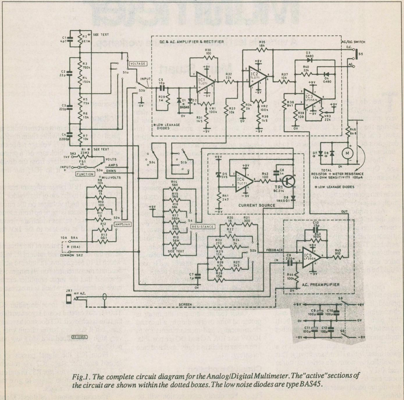
Fig.1. The complete circuit diagram for the Analog/Digital Multimeter. The "active" sections of the circuit are shown within the dotted boxes. The low noise diodes are type BAS45.
