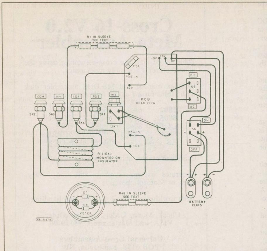
Fig. 4. Interwiring details for the off-board components. The circuit board and components are all mounted on the rear of the front panel. The series resistors are encased in plastic sleeving.
