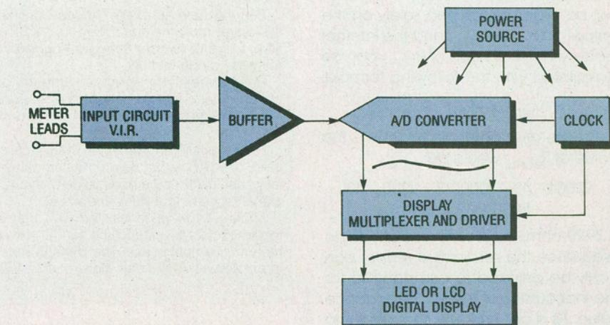
Fig. 6. This is a block diagram of a basic digital meter. The input circuit is programmed by the switches which are not shown here.
