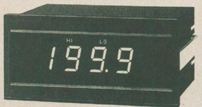
Here's a typical digital panel meter with an LED display. It requires front-end circuitry and switches to be really useful.
