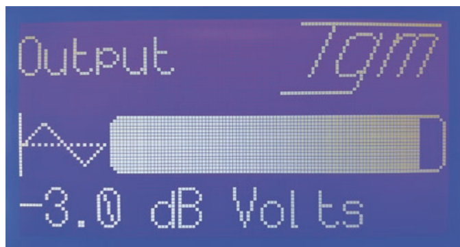
Screen 3: the next screen lets you set the output level from -123dBV (0.7mV RMS) to +5dBV (1.78V RMS) in steps of 0.1dBV.
