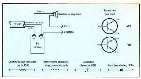
You can use your Thumb Thing to test components. Just connect the output (X) and ground (Y) leads across the components as shown. Transistors should be treated as two diodes, with the leads connects as shown for each diode junction.
