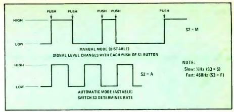
You can set your Thumb Thing to provide a continuous square wave output, as shown on the lower trace, of  $\frac{1}{2}$  or 460 Hz. You can also operate your Thumb Thing manually, as shown on the upper trace. When operated manually, the output state changes each time the pushbutton is depressed.
