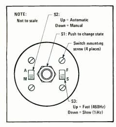
The mode and frequency slide switches are mounted beside the pushbutton using 2-56 machine screws and nuts.
