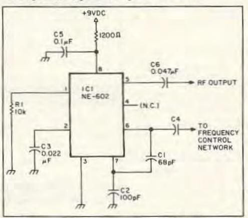
Figure 2. Generic NE-602 oscillator circuit.
