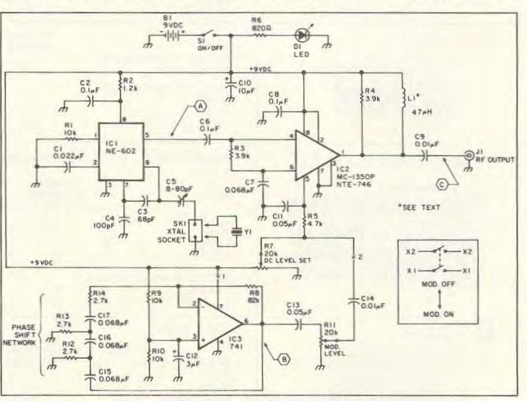
Figure 4. Circuit diagram for the signal generator.
