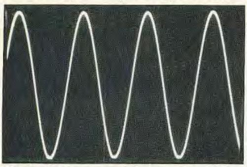
Photo C. Output waveform: AF from 741.
