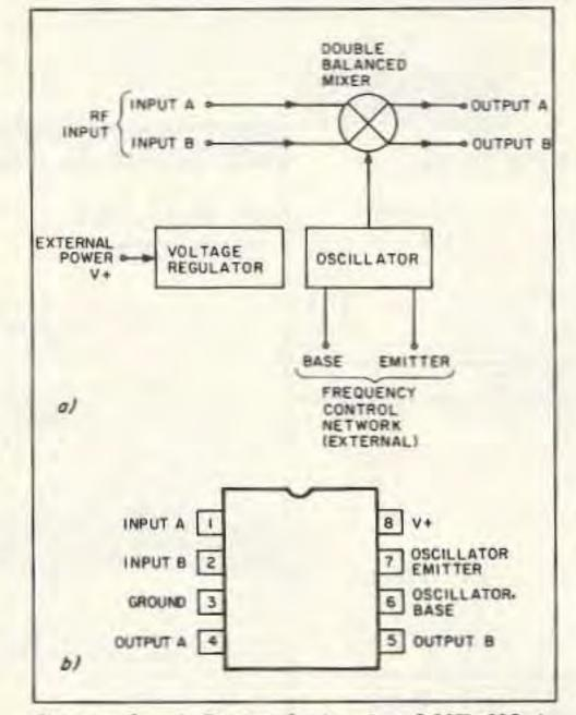
frequencies use a higher value. In general, the capacitor should be 0.001  $\mu$ F to 0.01  $\mu$ F for VHF, 0.01  $\mu$ F to 0.05  $\mu$ F for HF, and 0.05  $\mu$ F to 0.33  $\mu$ F for VLF through low HF frequencies.
