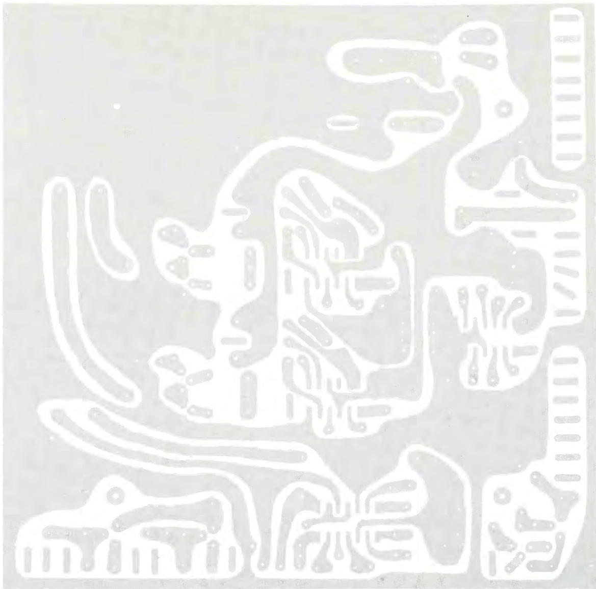
Fig. 4. Above is the actual-size etching-and-drilling guide; opposite page is components-placement diagram.
