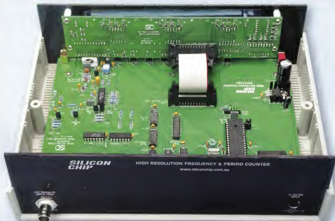
This is the view inside the completed 2.5GHz frequency counter, from the rear. All the parts fit on the main and display PCBs and these are linked together by a short IDC cable (see Figs.10 & 11). Power comes from a 9-12V DC 1A plugpack supply.
